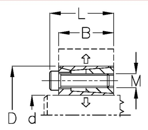
$\begin{array}{lll} \text{B mm} & = 28 \\ \text{d mm} & = 60 \\ \text{D mm} & = 88 \\ \text{Fit tolerance} & = \text{Aksel h8, Nav H8} \\ \text{F kN torque} & = 90 \\ \text{L mm} & = 36 \\ \text{M mm} & = \text{M8} \\ \text{P N/mm2 surface pressure on shaft/hub} = 100 \\ \end{array}$
